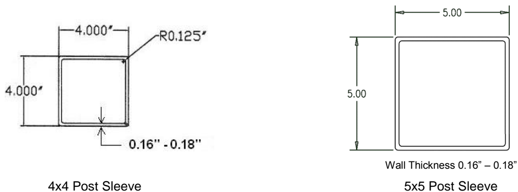
Figure 3 – TAM-RAIL® Post Sleeve Cross Sections
