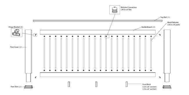
Figure 4 - Evolutions Rail™ / Builder with Steel Balusters
