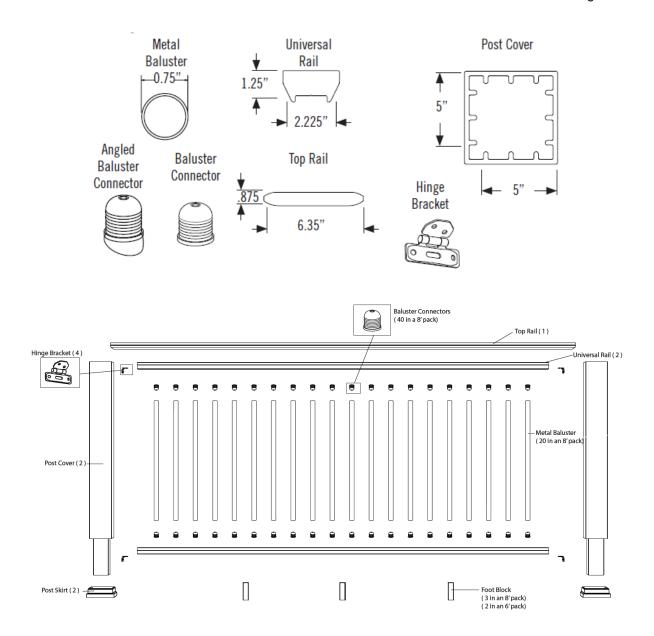
Figure 3 - Evolutions Rail™ / Contemporary with Steel Balusters
