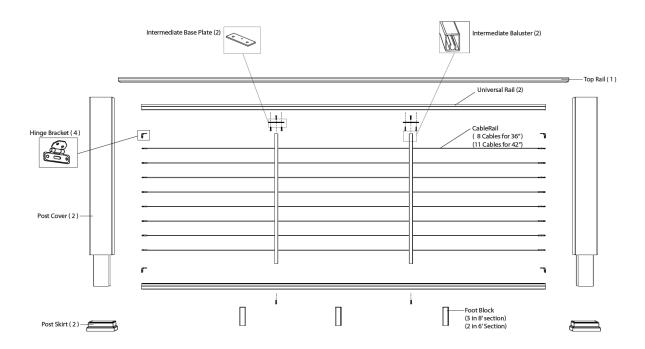
Figure 2 – Evolutions Rail™/ Contemporary with Feeney® CableRail®
