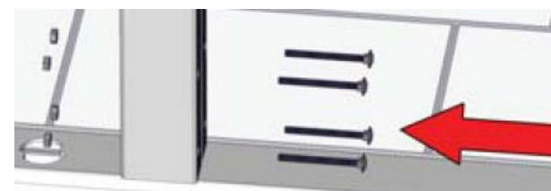
Post attachment to Post Bracket
