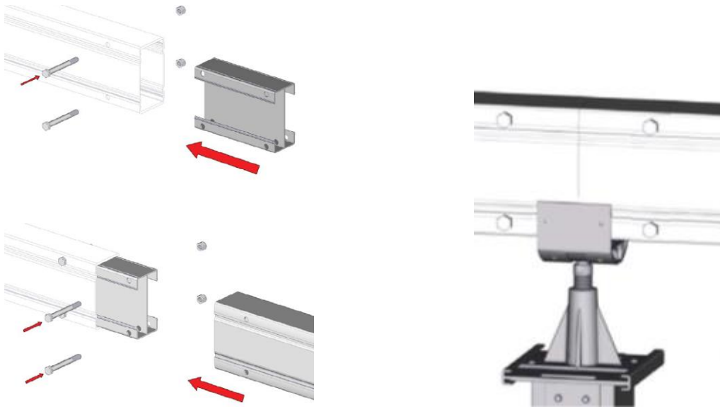
Figure 11 – Beam to Beam Connection
