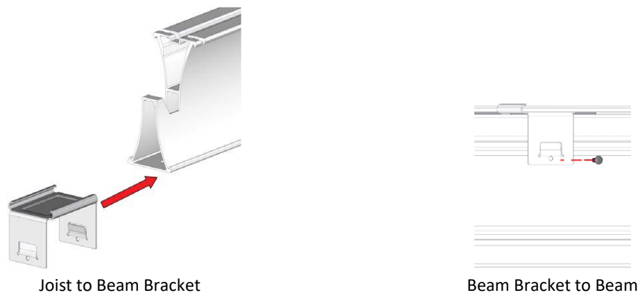
Figure 16 – Interior Joist to Beam
